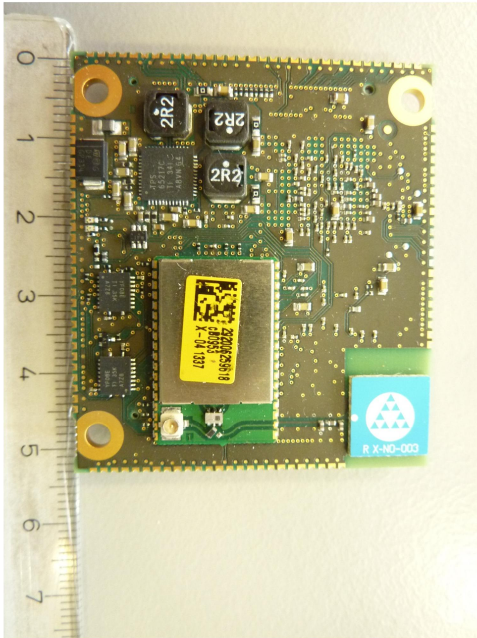
136117_DFS5.JPG: ODIN-W160 (TI-driver), soldered on CB-0960, top view
