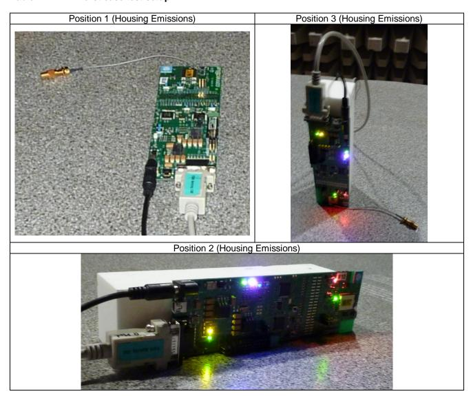
Preliminary tests were performed to find worst-case configuration and position. The radiated emission measurements were carried out in the orthogonal direction that emits the highest spurious emission levels.
