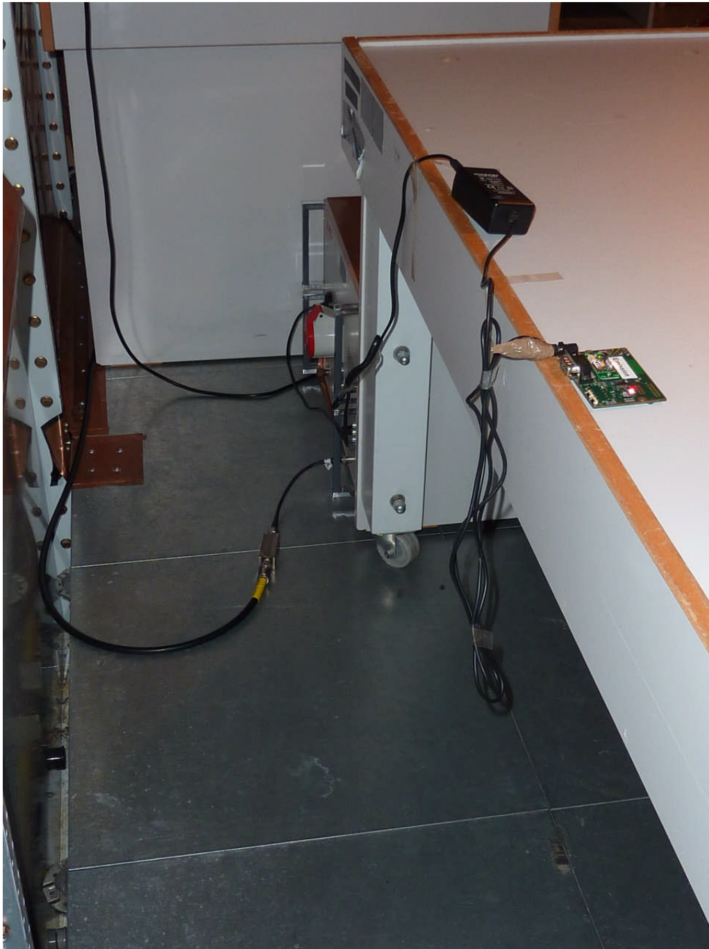
120262_29.JPG: cB-0950 with internal antenna, test set-up shielded chamber
