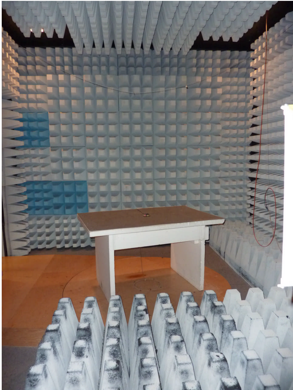
120262_3.JPG: cB-0950 with internal antenna (pos. 1), test set-up fully anechoic chamber
