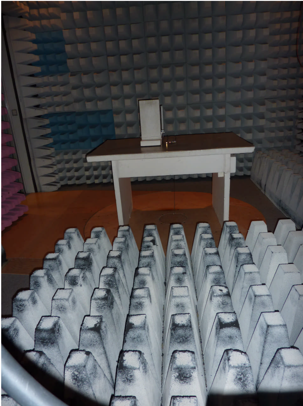
120262_15.JPG: cB-0950 with external monopole antenna (pos. 1), test set-up fully anechoic chamber
