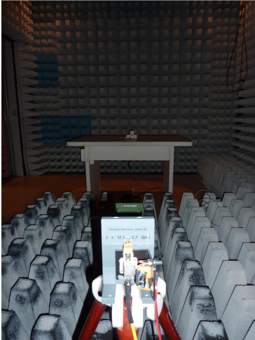
124266_4.JPG: Test setup fully anechoic chamber
