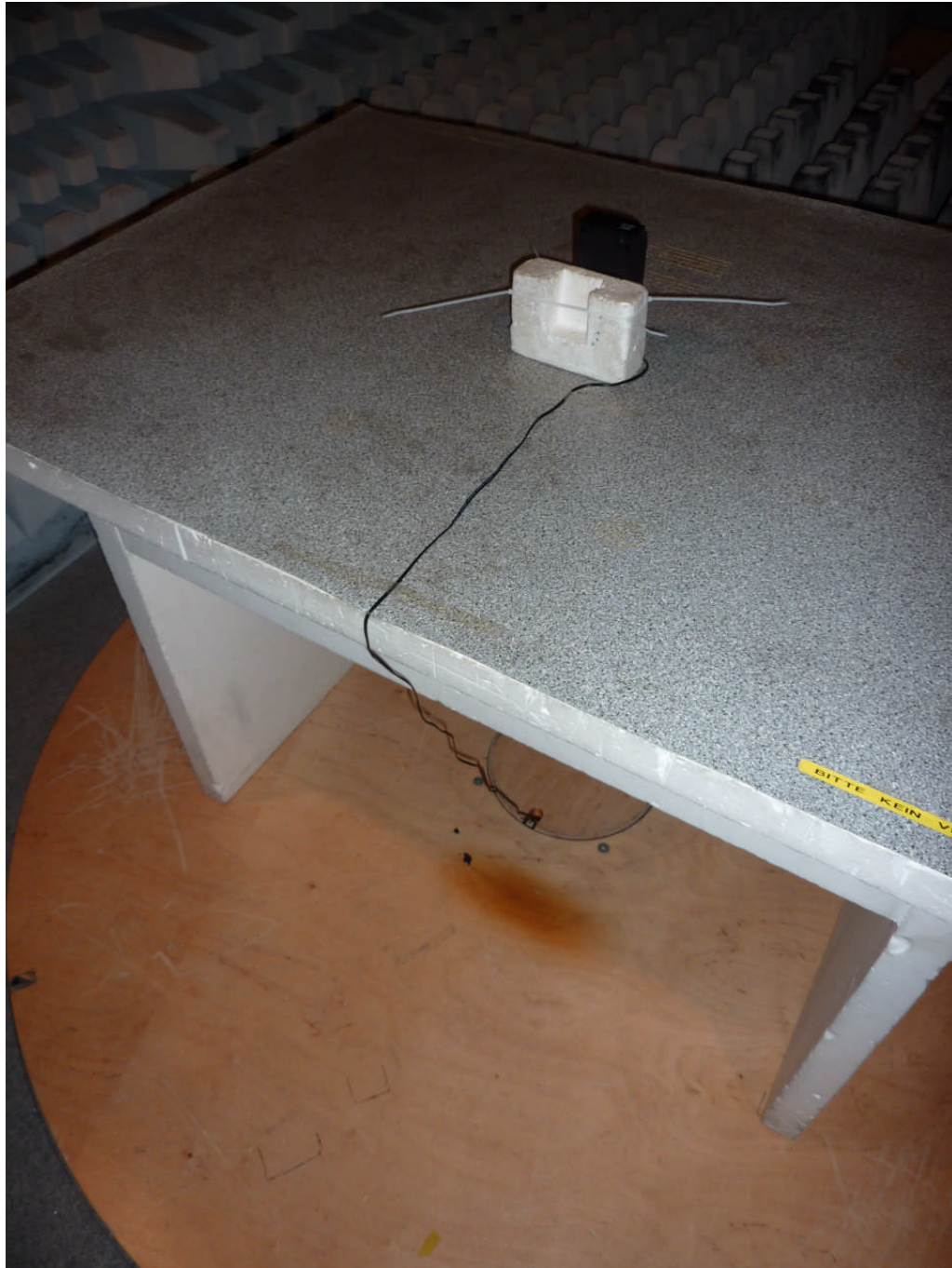
111592_26.JPG: cB-0946 with EPA antenna, test setup fully anechoic chamber (pos. 3)
