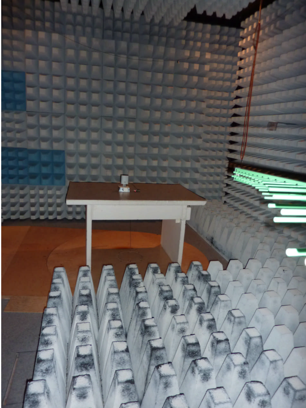
111592_15.JPG: cB-0946 with external patch antenna, test setup fully anechoic chamber
