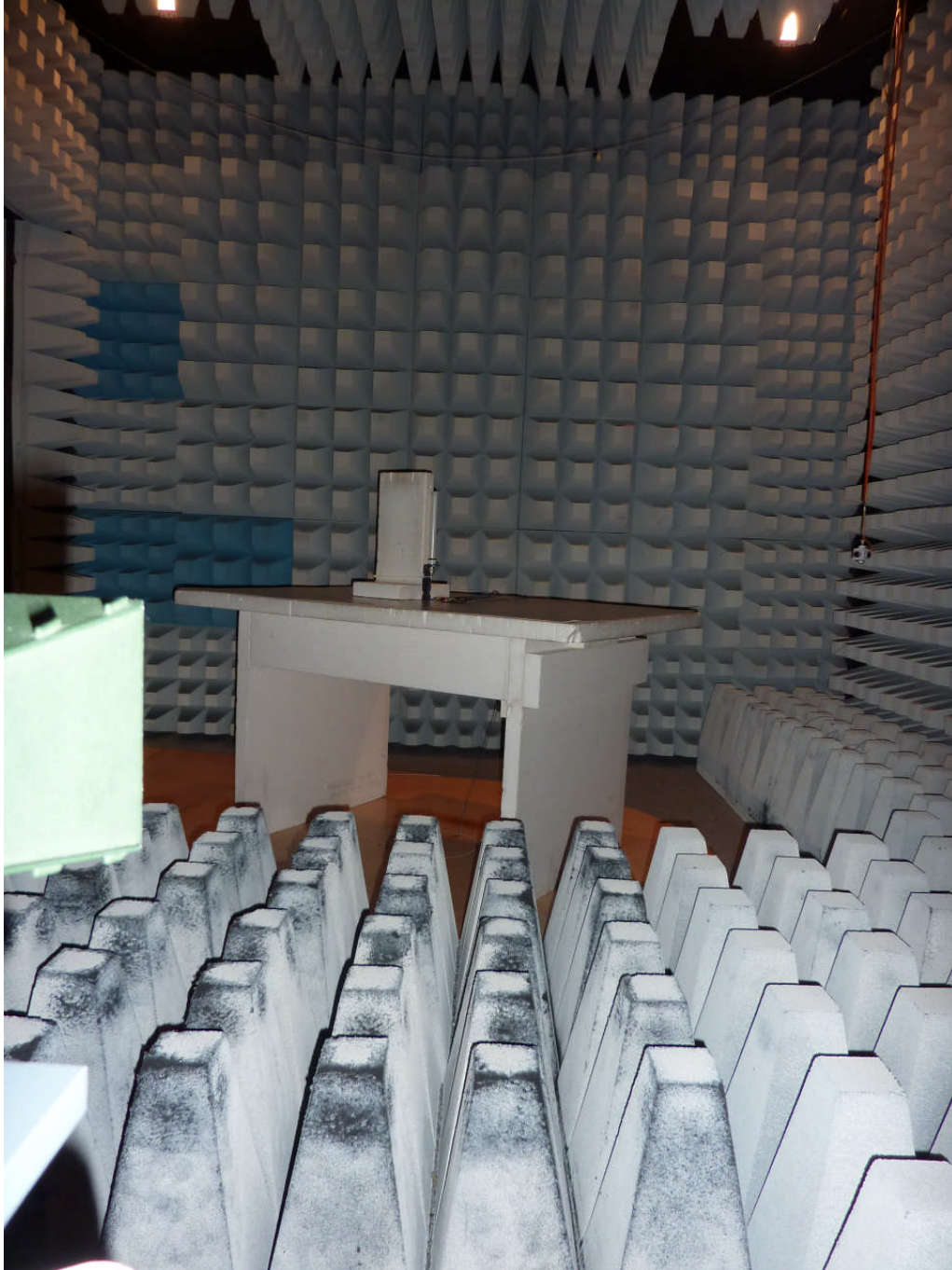
111592_19.JPG: cB-0946 with external monopole antenna, test setup fully anechoic chamber
