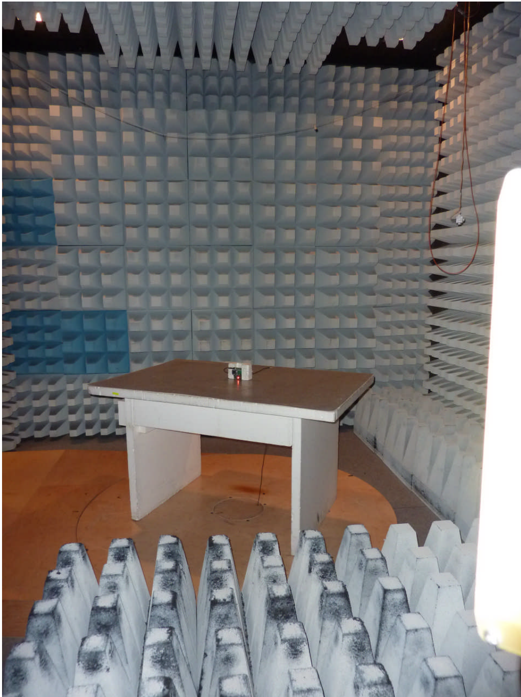
111592_40.JPG: cB-0946 with internal antenna, test setup fully anechoic chamber
