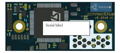
An auxiliary label will be provided for systems using the module where the original label not will be visible when the module is installed.
