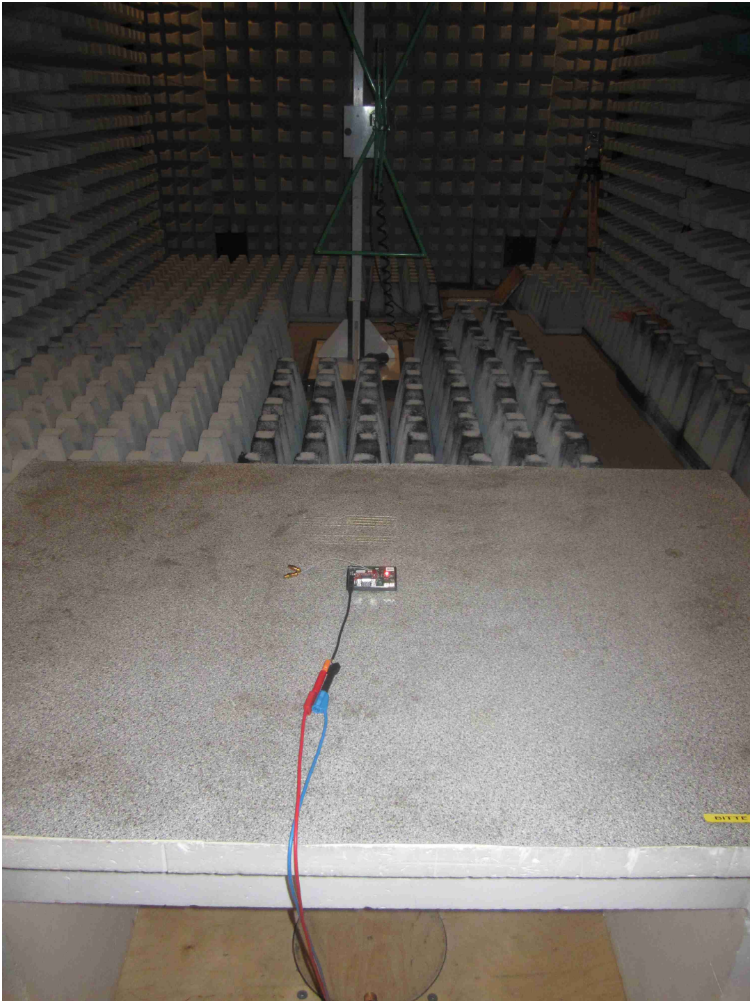
120198_01: Test setup - Radiated emission, Antennas terminated (fully anechoic chamber)
