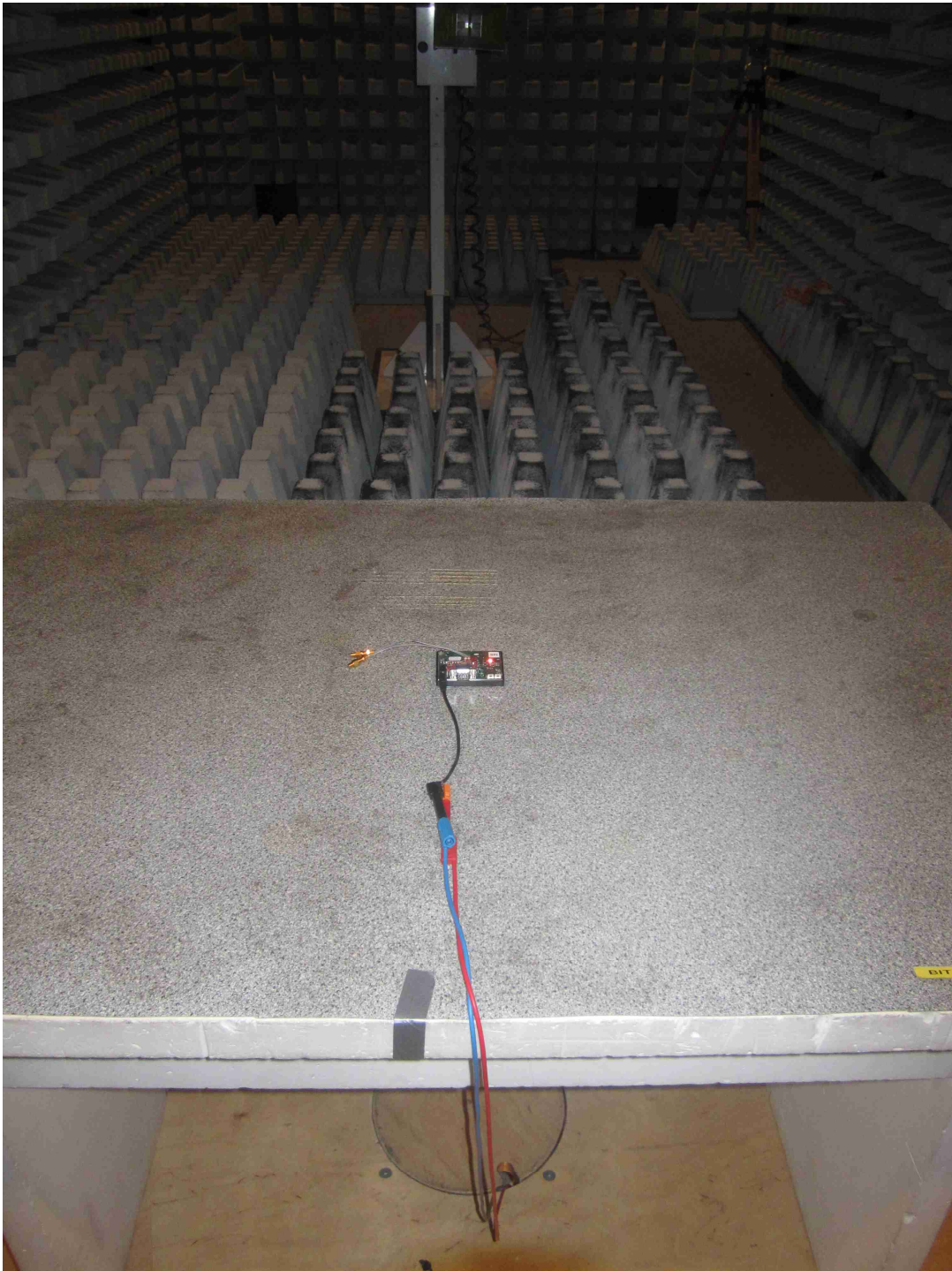
120198_02: Test setup - Radiated emission, Antennas terminated (fully anechoic chamber)
