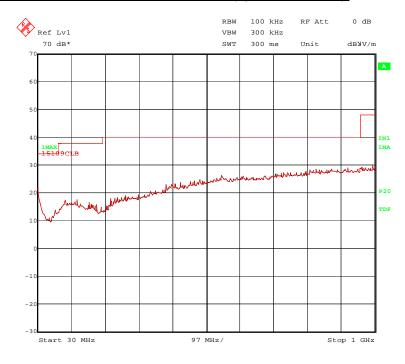
No emissions were found in the frequency band from 30 MHz to 1 GHz, therefore no final measurement on the open area test site was necessary.
