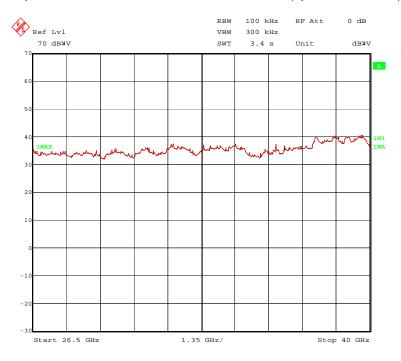
The following frequency was found inside the restricted bands during the preliminary radiated emission test:
