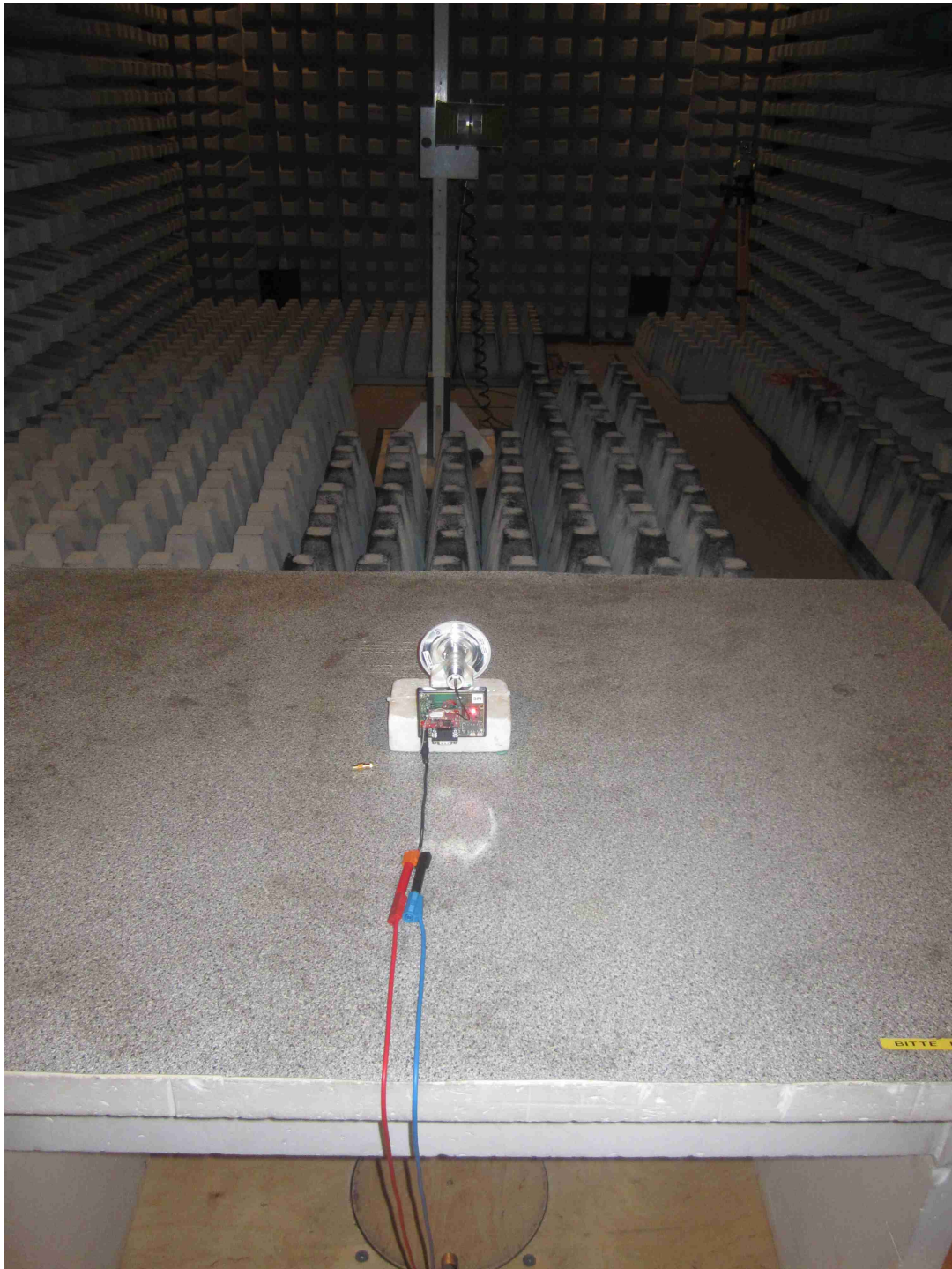
120198_04: Test setup - Radiated emission, Ant 2 (fully anechoic chamber)
