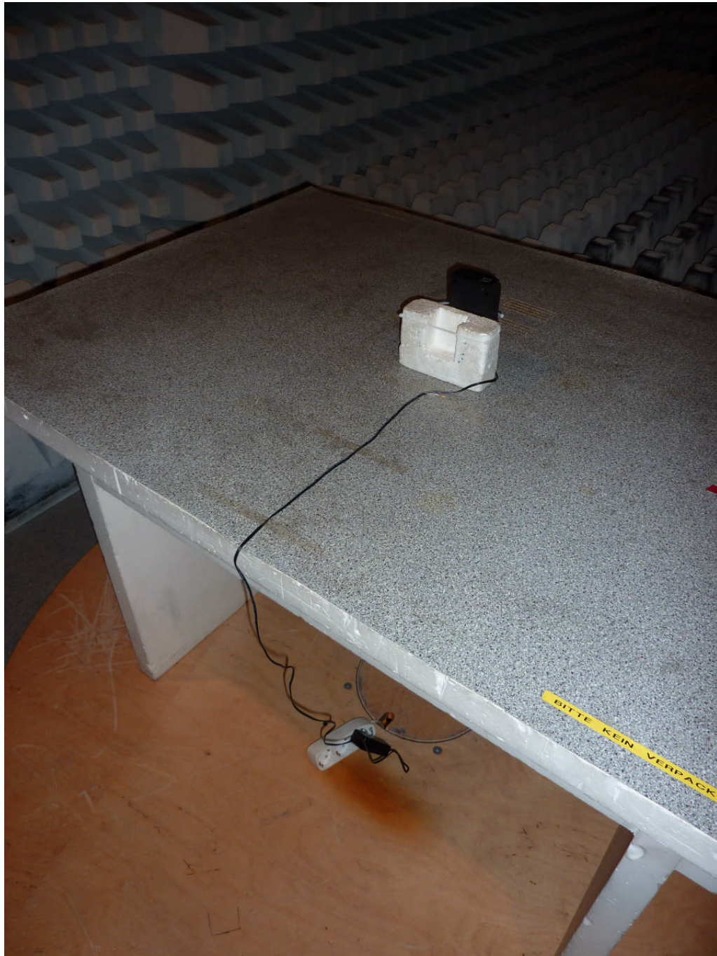
112117_2.JPG: cB-0939 with EPA antenna, test setup fully anechoic chamber
