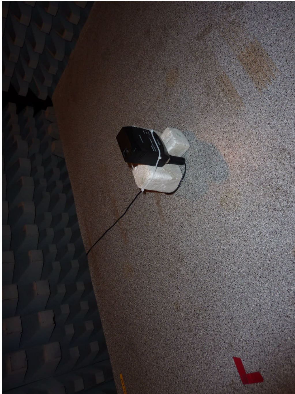
112117_3.JPG: cB-0939 with EPA antenna, test setup fully anechoic chamber
