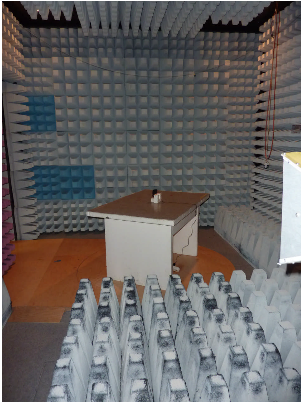
112117_1.JPG: cB-0939 with EPA antenna, test setup fully anechoic chamber
