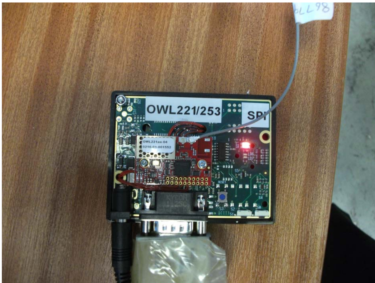
Photo #2. Conducted measurement setup. The red PCB is the connectBlue module. The green PCB is the OEM Module Adaptor. The grey cable is the RF cable connected to the transmitter RF port.
