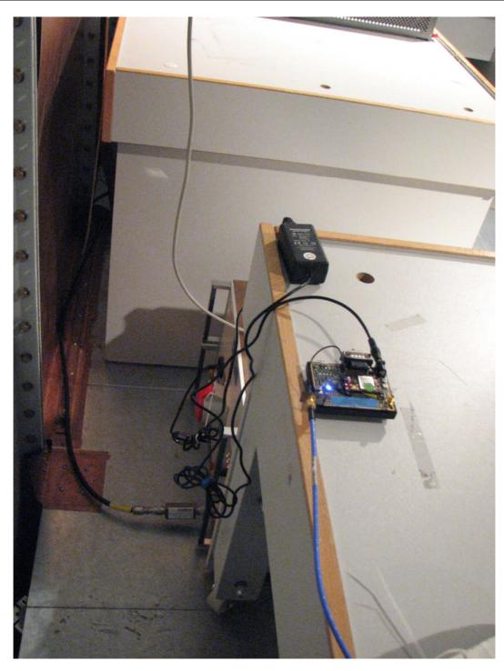
72323\_3.jpg cB-OWLAN211gx-02 test set-up conducted emission measurement
