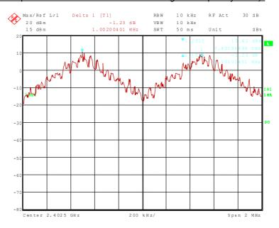
72194\_112.wmf: (channel separation at the middle of the assigned frequency band):
