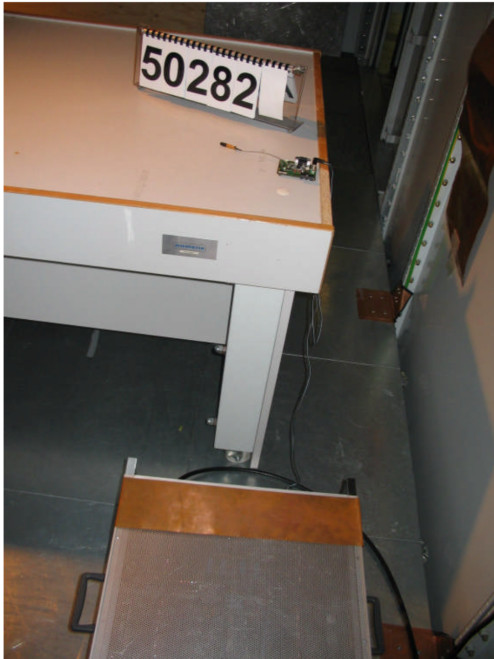
50282cemi1.jpg cB-0719-02 test set-up conducted emissions
