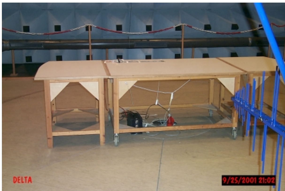
PHOTO A2.2 Test set-up for test 30-1000 MHz
