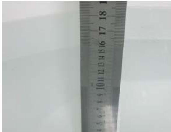
Liquid Height for Body SAR
