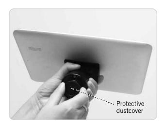
**Step 1:** Unscrew the protective dust cover from the bottom of the Moticam T2 to expose the imaging sensor to light.
