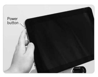
**Step 4:** Press and hold the power button for 2-3 seconds to boot up the Moticam T2.
