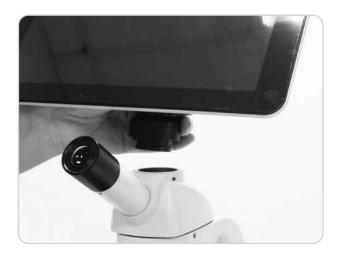
**Step 2:** Mount the Moticam T2 onto your microscope's C-mount, and if your microscope is equipped with a beam splitter, pull the beam splitter to ensure light can reach to the trinocular port.
