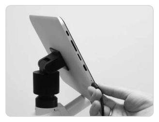
**Step 3:** Plug in the Moticam T2 power supply and press the power button to start.
