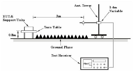
The radiated emission tests were performed in the 3 meters chamber test site, using the setup accordance with the ANSI C63.4-2003. The specification used was the FCC Part 15.109, Class B limits.
