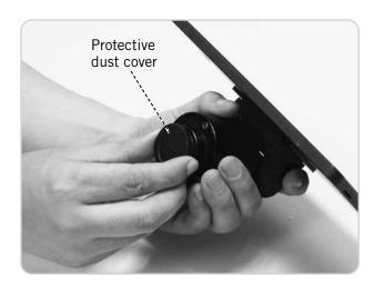
**Step 1:** Unscrew the protective dust cover from the bottom of the Moticam S2 to expose the imaging sensor to light.
