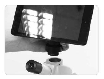
**Step 2:** Mount the Moticam S2 onto your microscope's C-mount, and if your microscope is equipped with a beam splitter, pull the beam splitter to ensure light can reach to the trinocular port.
