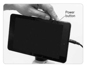
**Step 4:** Press and hold the power button for 2-3 seconds to boot up the Moticam S2.
