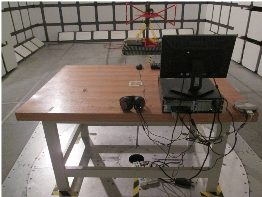
Radiated Emissions – Rear View (30-1000 MHz)
