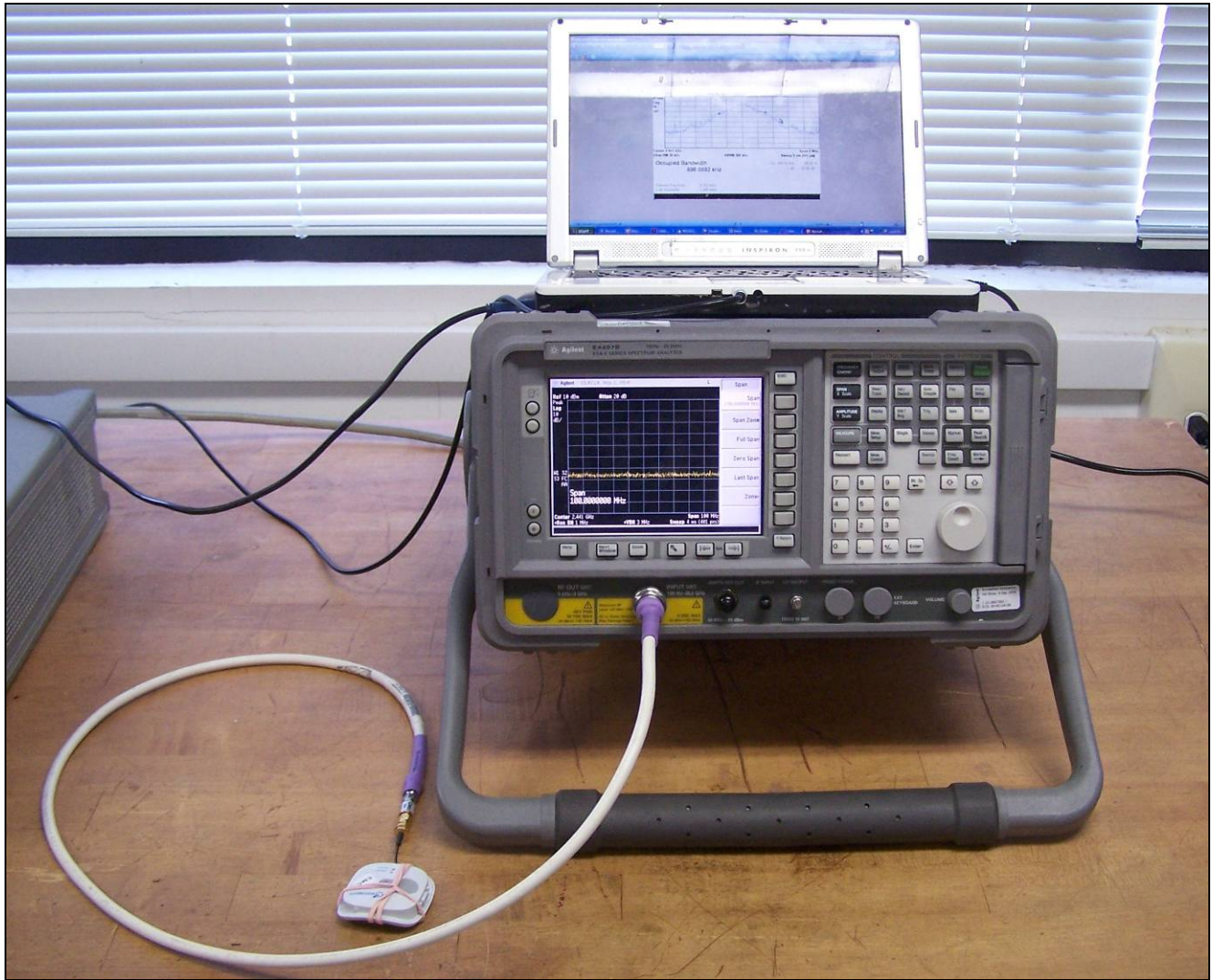
Photograph 5. Conducted Power, Test Setup
