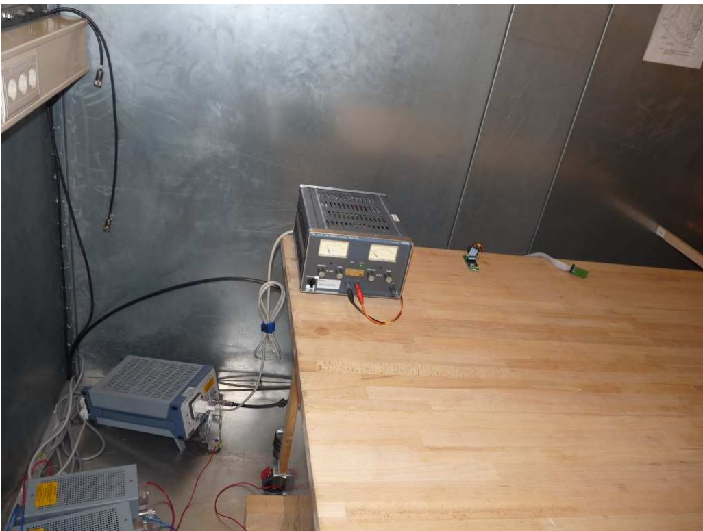
Photo 5: Test setup for conducted measurements (below 30 MHz, AC mains)
