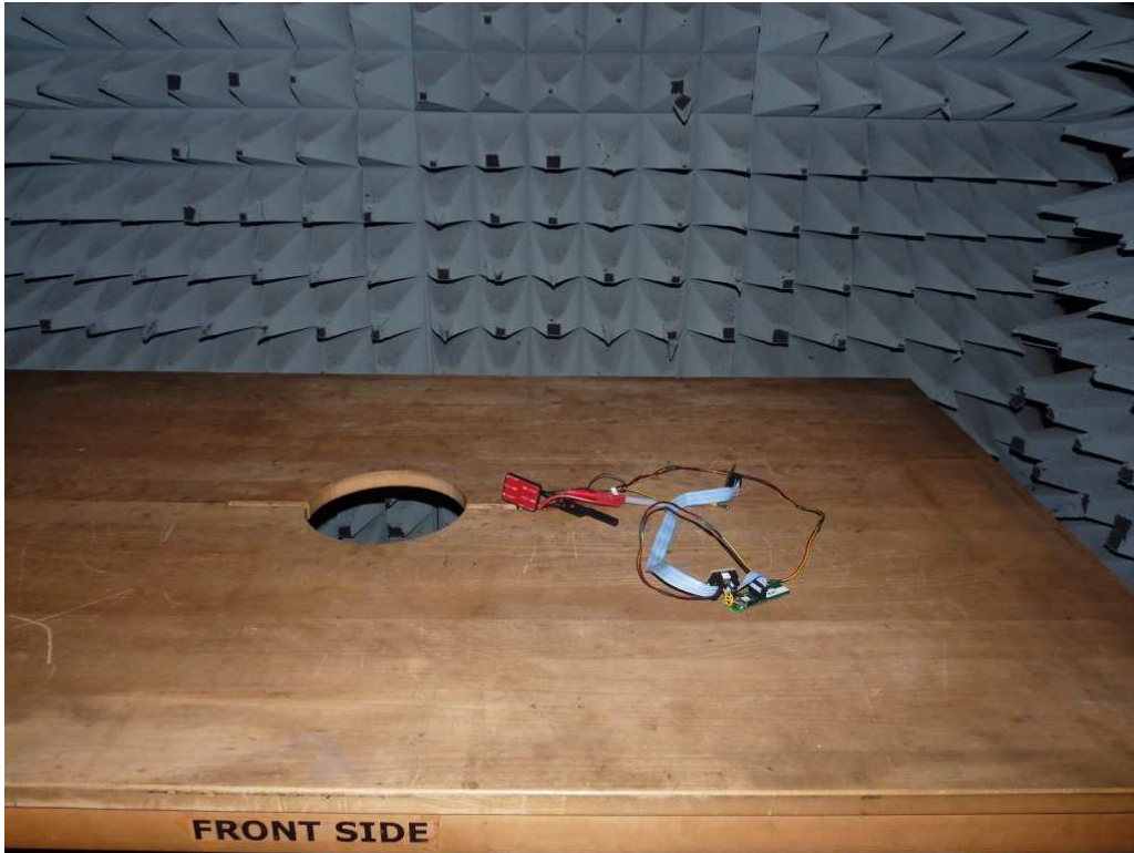
Photo 1: Test setup for radiated measurements (below 30 MHz)
