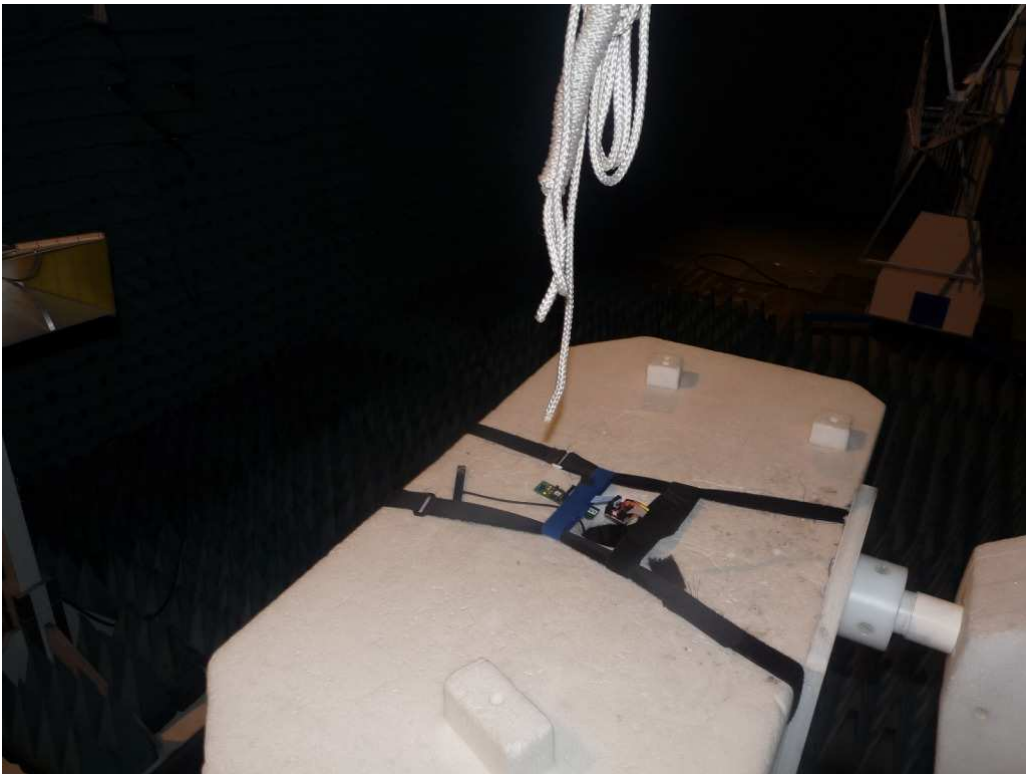
Photo 3: Test setup for radiated measurements (above 1 GHz up to 18 GHz)
