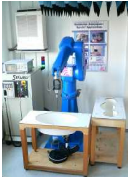
Fig. 4: The measurement set-up with a DASY system and phantoms containing tissue simulating liquid.
