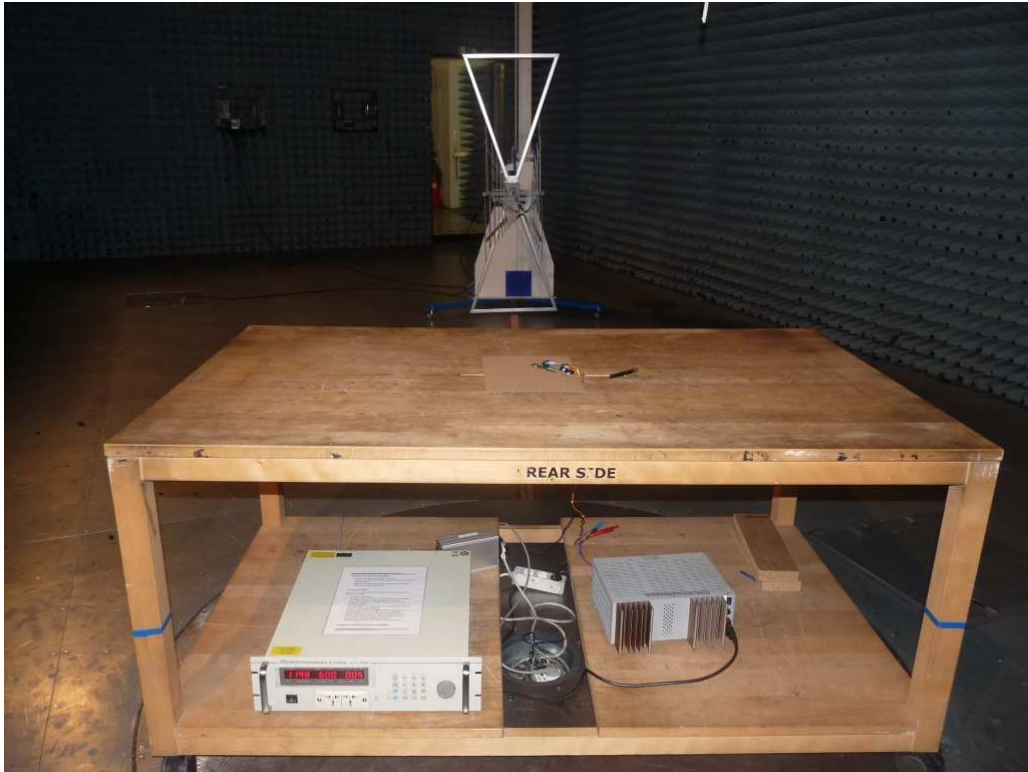
Photo 2: Test setup for radiated measurements (30 MHz to 1 GHz)
