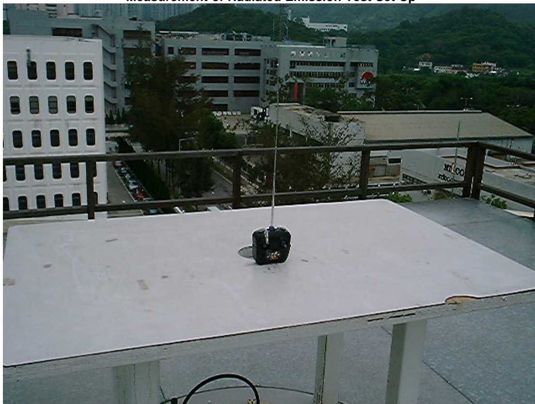
Measurement of Radiated Emission Test Set Up
