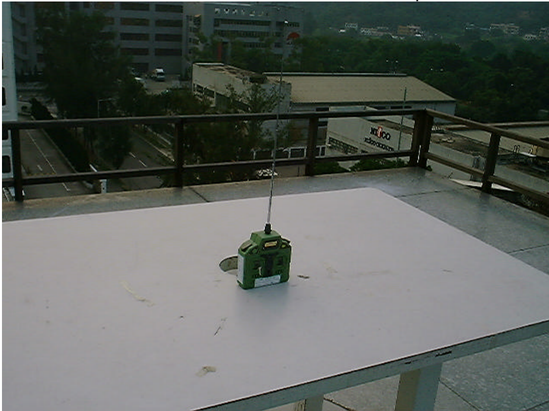
Measurement of Radiated Emission Test Set Up
