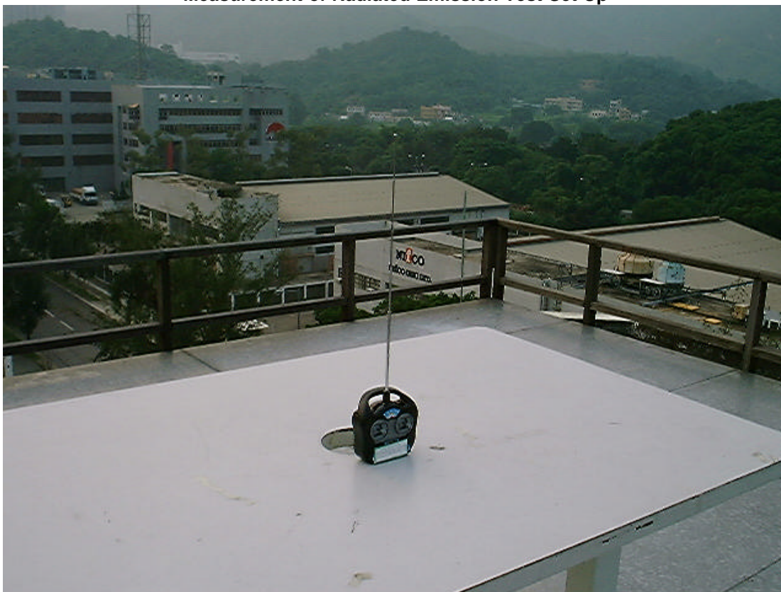
Measurement of Radiated Emission Test Set Up
