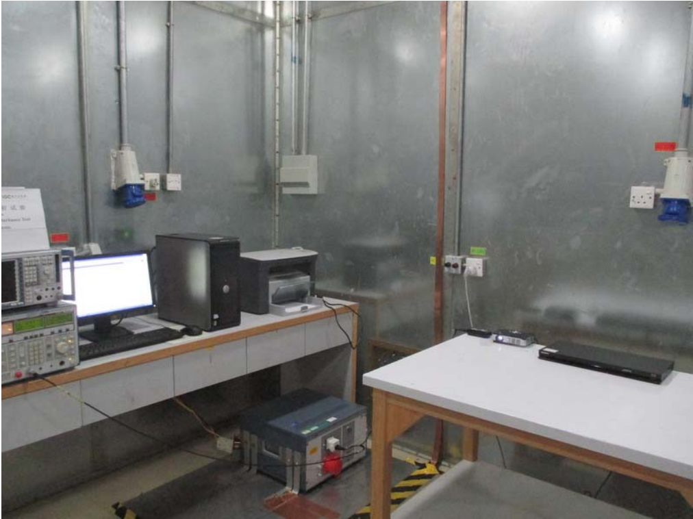
FCC RADIATED EMISSION TEST SETUP
