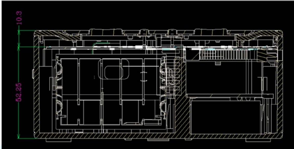
The minimum contact distance is 10.3 mm. So, the 10mm separation distance applies.
