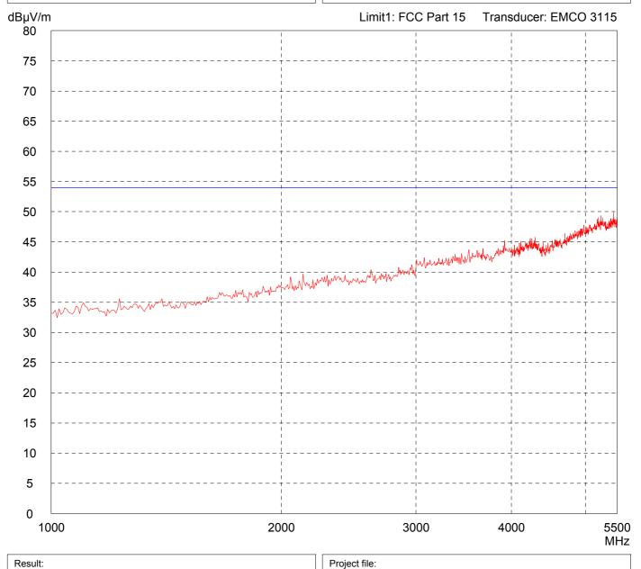
Model: 70RX-S1 Serial no.: Sample 1 Applicant: HM-Funktechnik GmbH Test site: Fully anechoic room, cabin no. 2 Tested on: Test distance 3 metres Vertical Polarization Date of test: Operator: 09/03/2004 T. Eberl File name: Test performed: automatically default.emi
