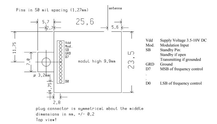
D0 to D7 changes the frequency of the transmitter. If the pins D0 to D7 are all open the transmitter works with the lowest programmed frequency. The frequency adjustment is digitally coded. Grounding of D0 rises the frequency about the channel spacing 25KHz. D1 rises about double D0, D2 rises about double D1 and so on. So D7 rises the frequency about 1600 times of D0  $(2^7)$ , that means 3.2MHz with 25KHz spacing.
