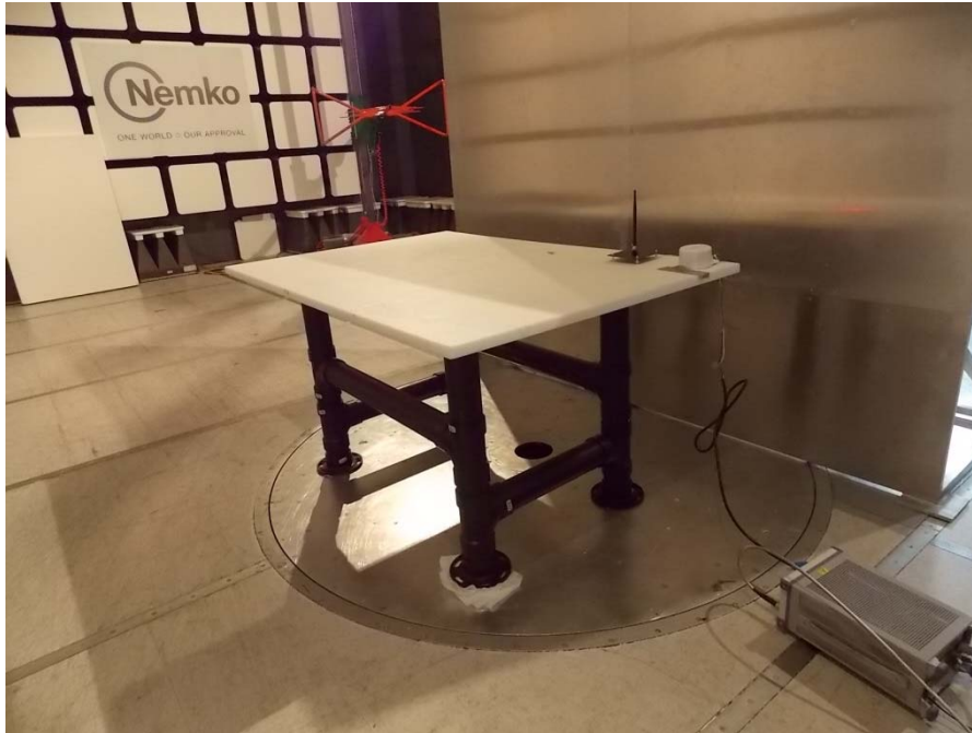
AC power line conducted emissions limits setup photo
