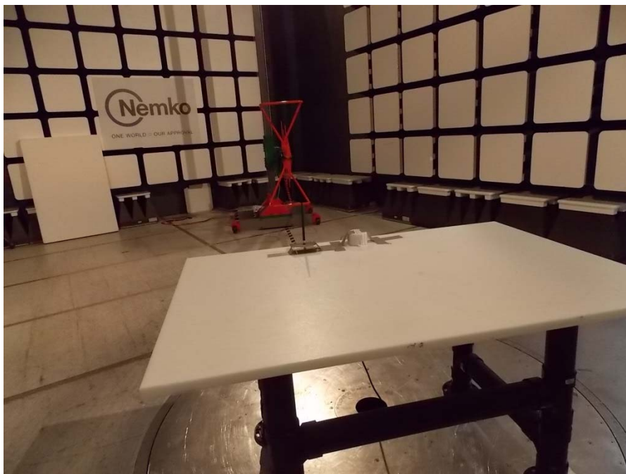
Radiated spurious (out-of-band) emissions setup photo – 30 to 1000 MHz
