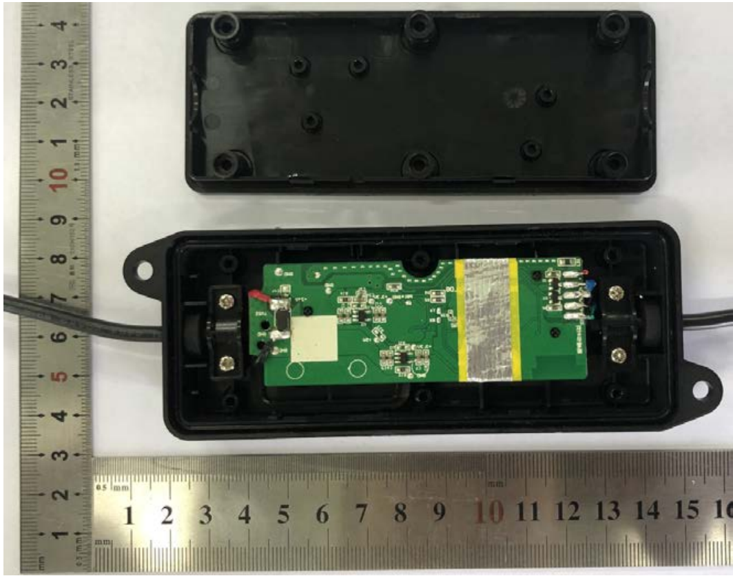
FIGURE 2 CYNC DIRECT CONNECTED OUTDOOR PREMIUM LIGHT STRIP (32FT.) (M/N: CLEDSTR36LCDODP) MAIN BOARD FRONT
