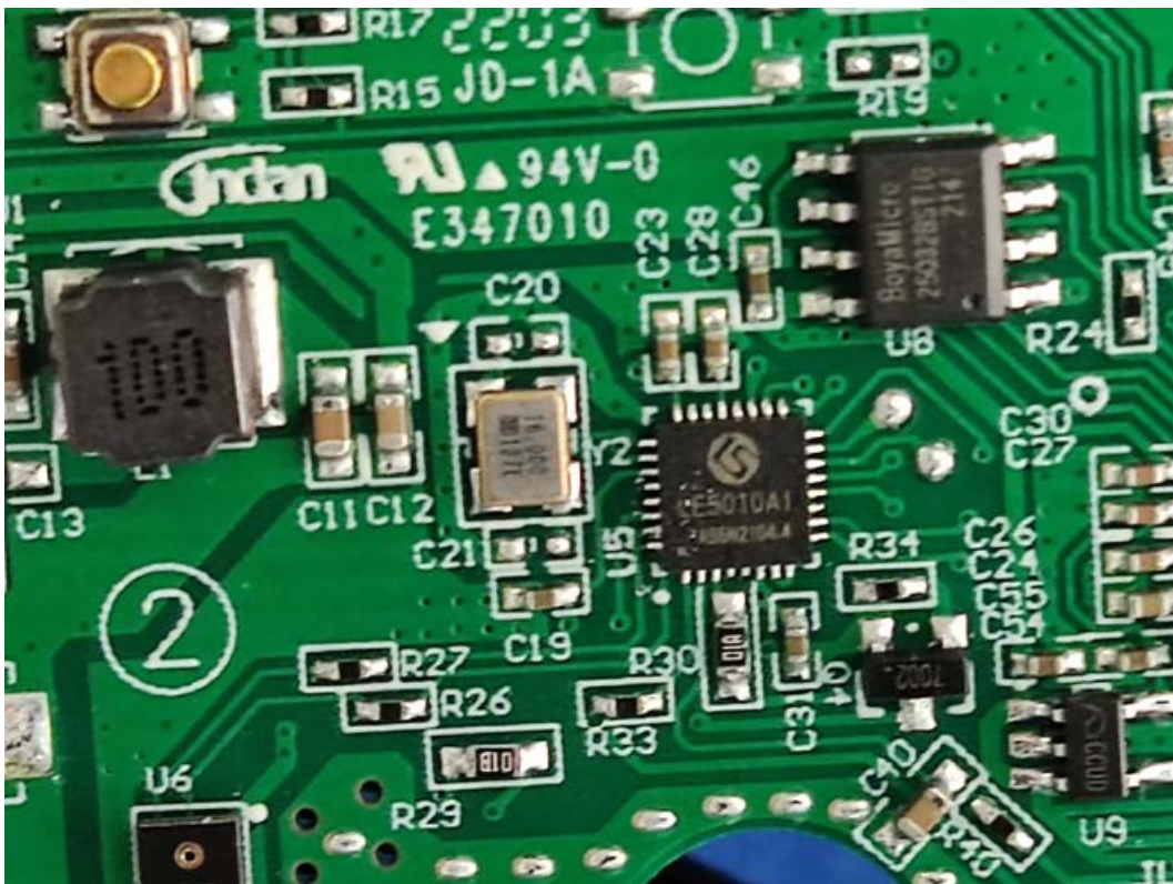
FIGURE 4 CYNCR DIRECT CONNECTED OUTDOOR PREMIUM LIGHT STRIP (32FT.) (M/N: CLEDSTR36LCDODP) CHIP & CRYSTAL ON RBOARD
