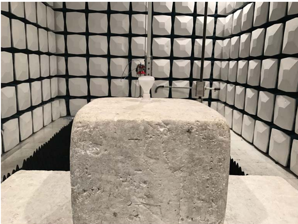
Description: Radiated Emission Test Setup for 1~18GHz
