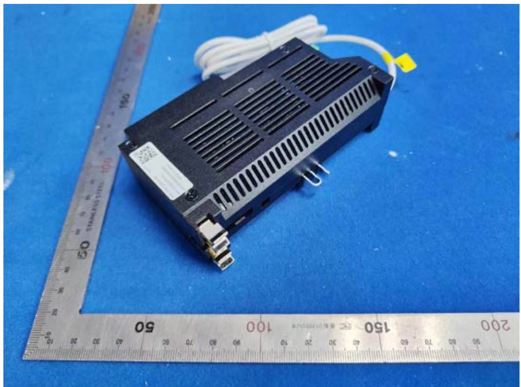
FIGURE 9 QO 2-CHANNEL POWER MONITOR MODULE, PIGTAIL (M/N: GPM-Q2SEM-00) GENERAL APPEARANCE BACK VIEW
