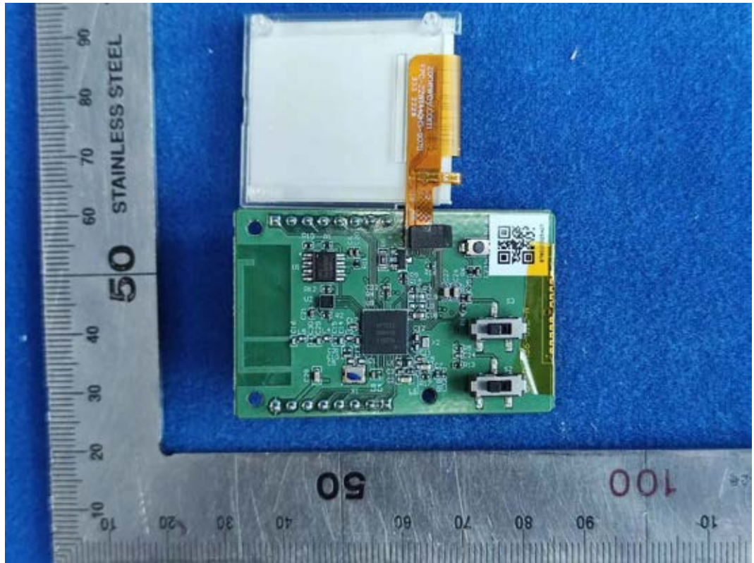
FIGURE 6 1-INCH 2-CHANNEL POWER MONITOR MODULE, PIGTAIL (M/N: GPM-H2SEM-00) RF BOARD BACK VIEW
