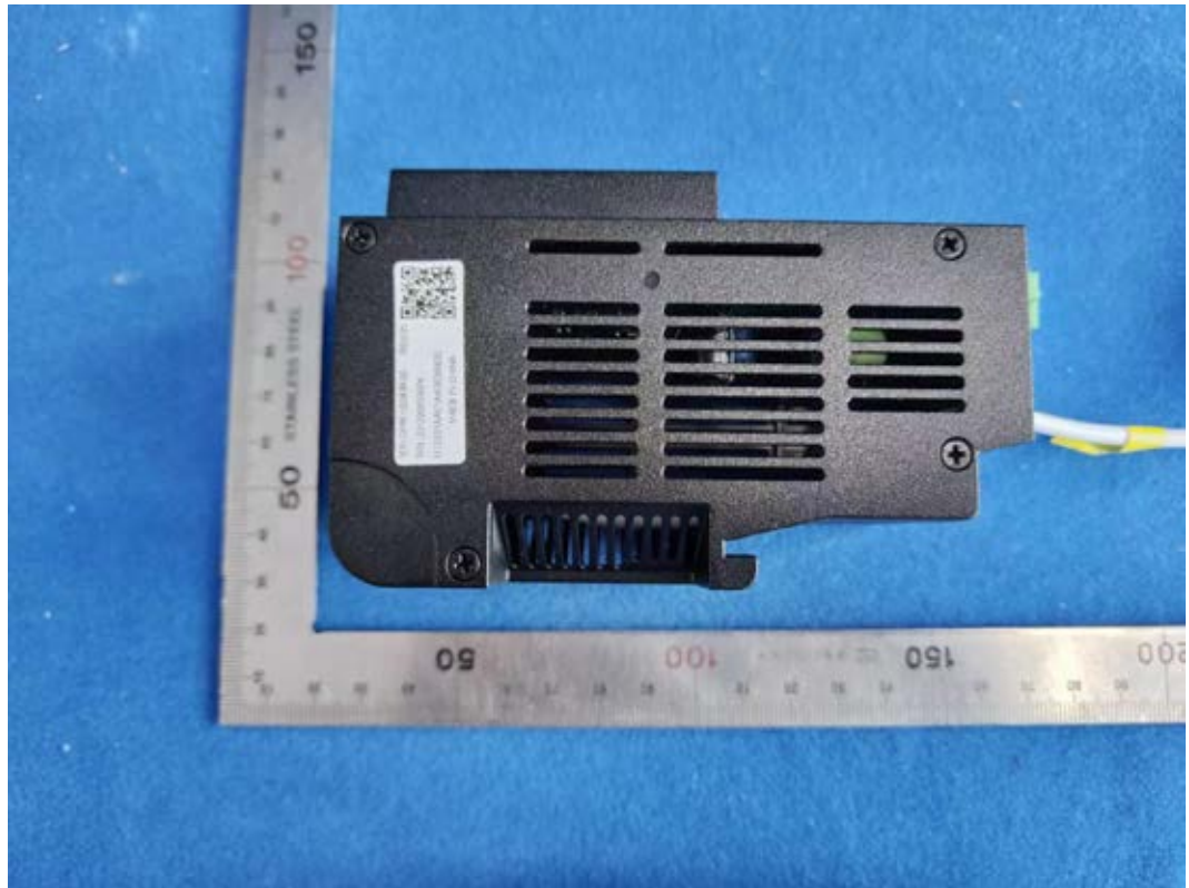
FIGURE 7 1-INCH 2-CHANNEL POWER MONITOR MODULE, PIGTAIL (M/N: GPM-H2SEM-00) GENERAL APPEARANCE BOTTOM VIEW
