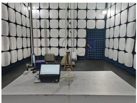
3. Radiated emission (9KHz-30MHz)
