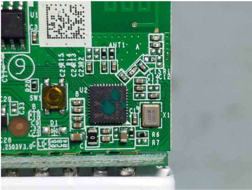
FIGURE 7 SMART PLUG (M/N: CPLGSTDBLW1) CHIP & CRYSTAL ON RF BOARD (GENERAL VIEW)
