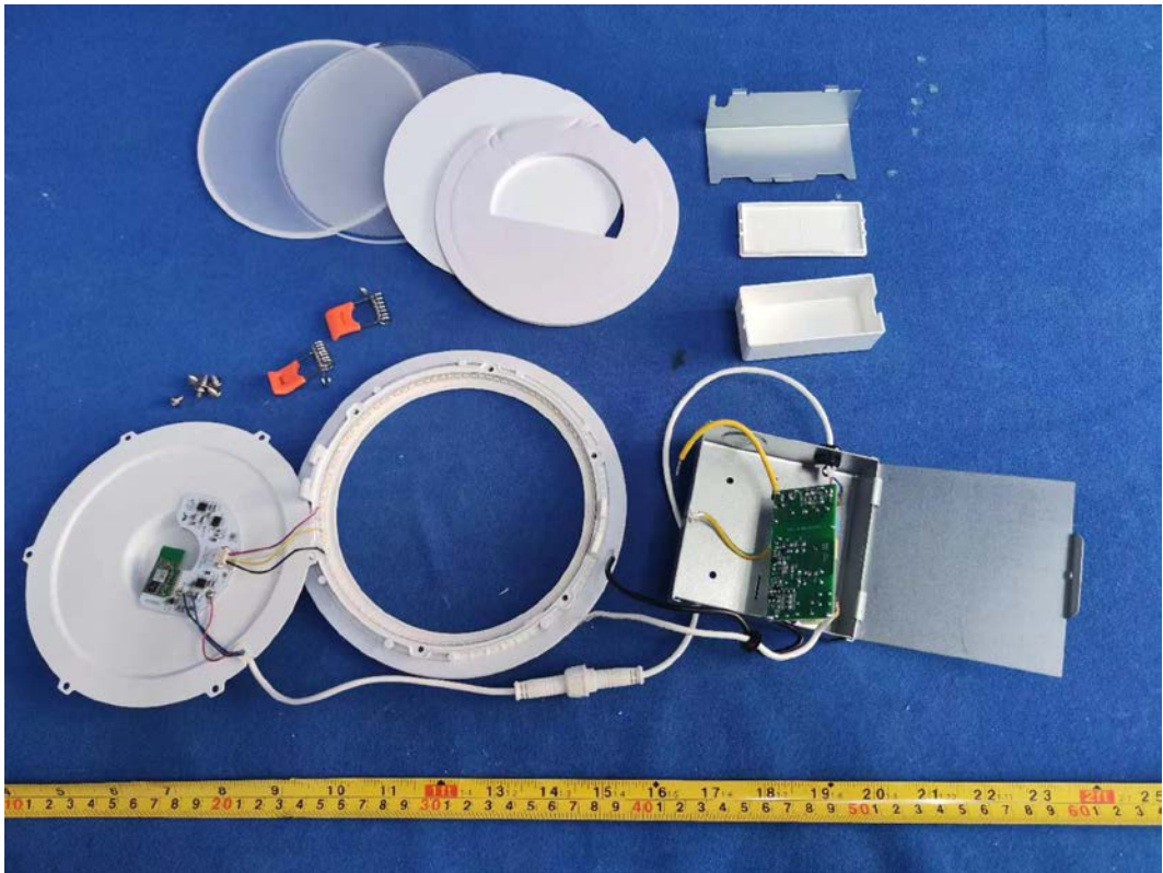
FIGURE 12 DOWNLIGHT (M/N: CFIXCNLR6S1) COVER REMOVED
