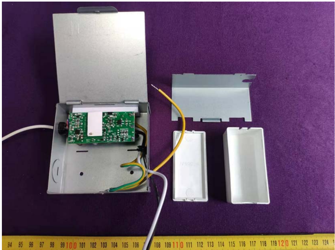
FIGURE 1 CYNC FIXTURE CANLESS (M/N: CFIXCNLR6S1) COVER REMOVED #1
