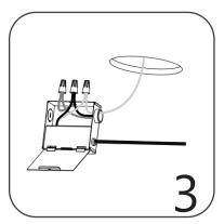
Bring the supply power to junction box through knockout and secure with strain relief. Use the wire nuts to connect power supply wires to respective color wires in the junction box.
