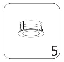
Hold the spring clips against the fixture and gently guide into the ceiling until the clips snap into place.
