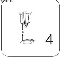
Place the junction box on the ceiling through cur hole. Connect the light with junction box with the connector.
