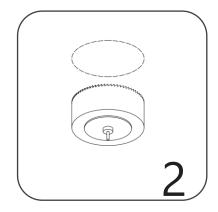
Drill hole in ceiling and prepare supply wire. Hole size CFIXCNLR4S1/ CFIXCNLR4C1 4 <sup>1</sup>/<sub>4</sub> inch, CFIXCNLR6S1/ CFIXCNLR6C1 6 <sup>1</sup>/<sub>4</sub>/inch.
