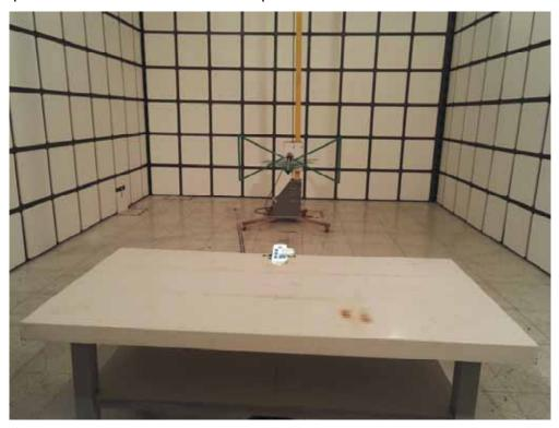
Description: Radiated Emission Test Setup for 1~18GHz
