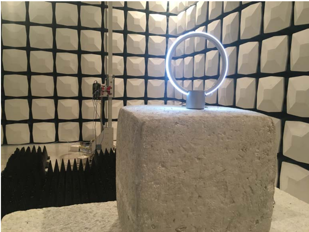
Description: Radiated Emission Test Setup for 1~18GHz
