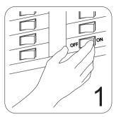
Turn off power source to the power supply where you are installing the fixture.
