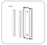
Apply adhesive tape to the groove of the faceplate bracket's back. Then mount the bracket to the wall.
