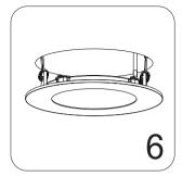
Hold the spring clips against the fixture and gently guide into the ceiling until the clips snap into place.
