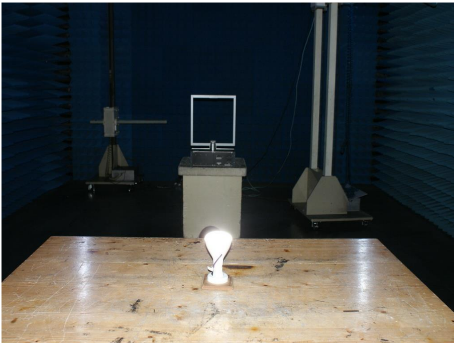
Photograph 4: Set-up for Radiated Spurious Emission, 9KHz - 30MHz
