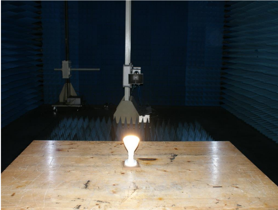
Photograph 4: Set-up for Radiated Spurious Emission, 9KHz - 30MHz
