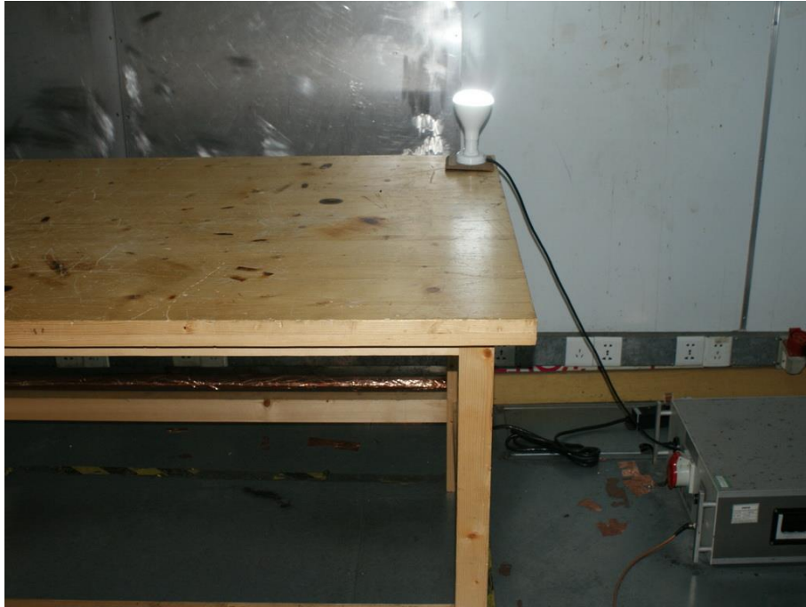
Photograph 1: Set-up for Conducted Emission on AC Mains
