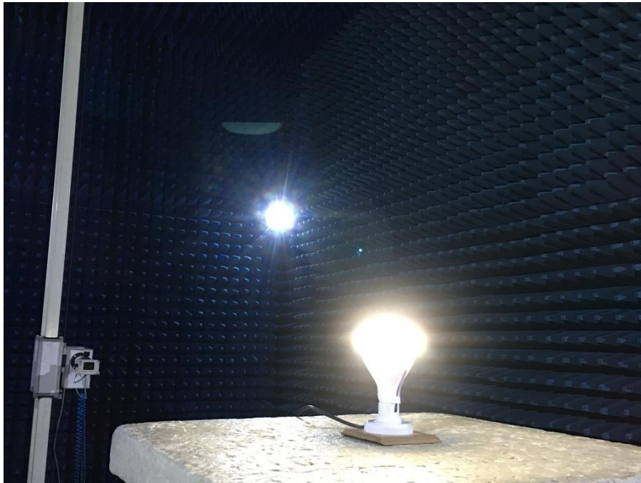
Photograph 7: Set-up for Radiated Spurious Emission, 18GHz - 26.5GHz
