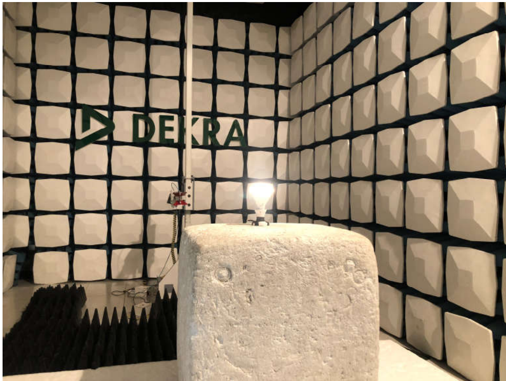
Description: Radiated Emission Test Setup for 1~18GHz
