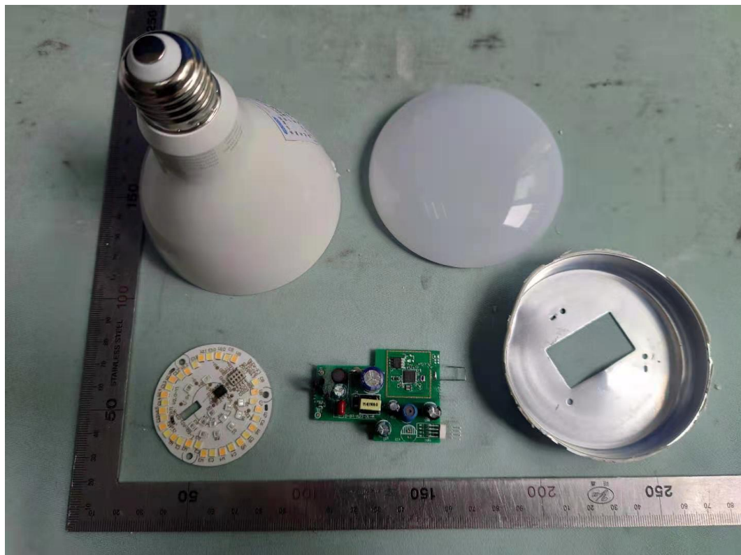
FIGURE 2 DUAL MODE FULL COLOR BR30 (M/N: CLEDR309CD1) GENERAL APPEARANCE (COVER REMOVED)
