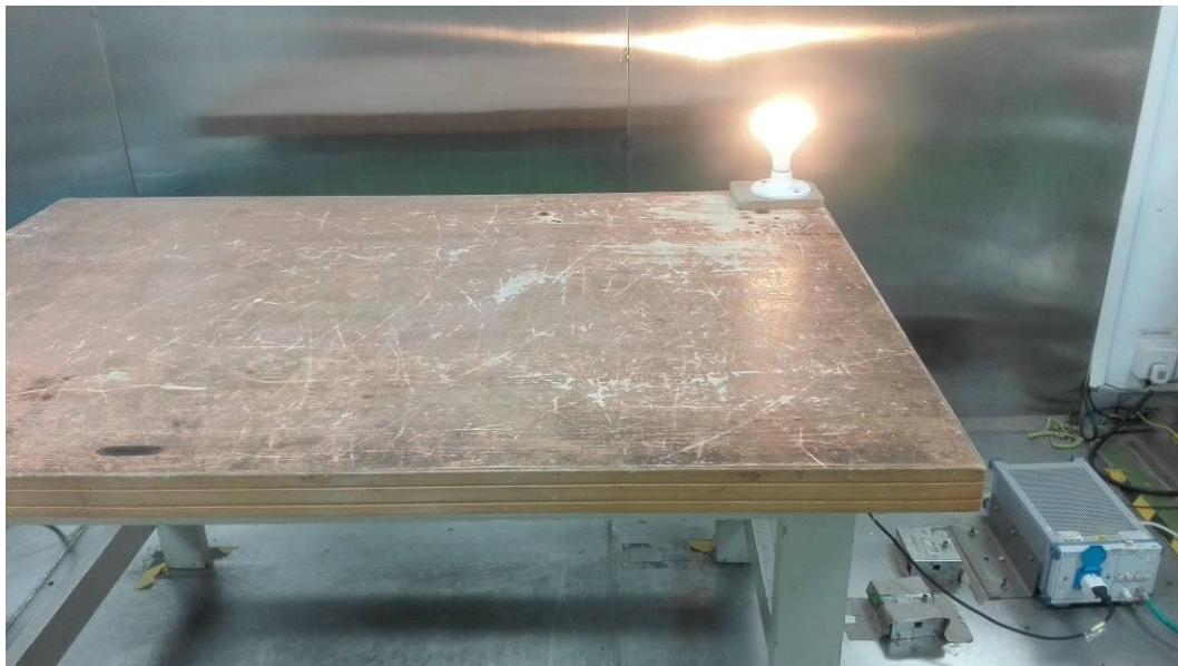
Conducted Emissions - Front View
