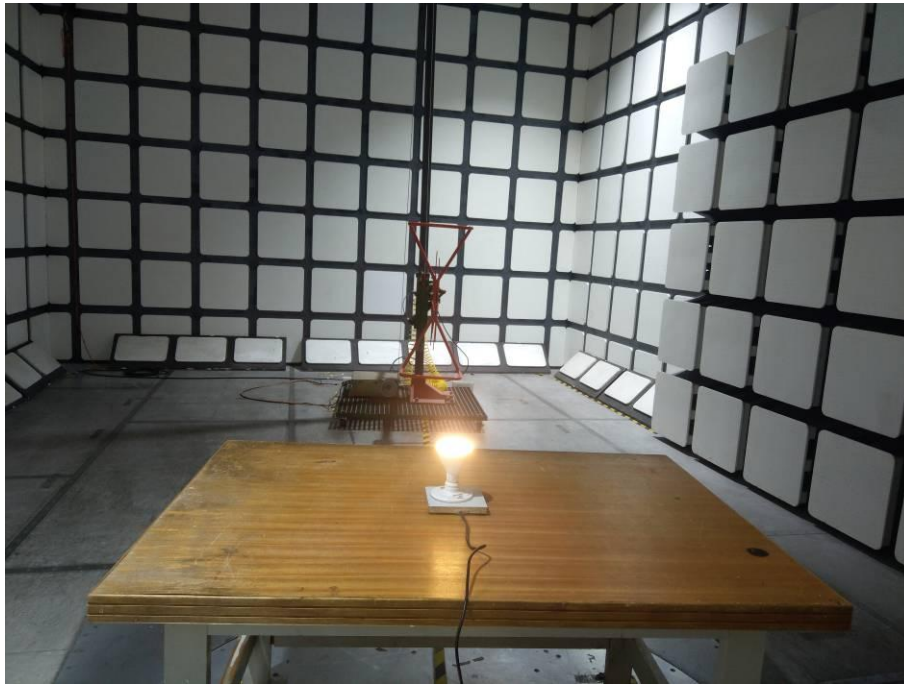
Radiated Emissions View (Below 1 GHz)
