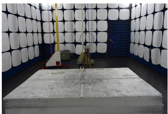
3. Radiated emission (9KHz-30MHz)
